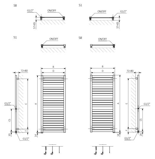
A - Height B - Width C1-C5 - Distance between pipe centres D - Horizontal distance between mounting bracket centres E - Vertical distance between mounting brackets F - Distance between a mounting bracket and the bottom of the radiator
